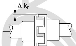
It compensates angular, radial and axial shaft misalignment within specified tolerances.
